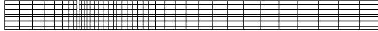
Fig. 4. A typical computational domain which has been employed in this study. It consists of 40 \times 7 \times 4 cells in the downstream, cross and vertical directions of the channel. This represents a mesh which is four times coarser in all three directions than the finest mesh used, namely, 160 \times 28 \times 16 , which contains 160 \times 28 \times 16 ( x, y, z ) cells.
